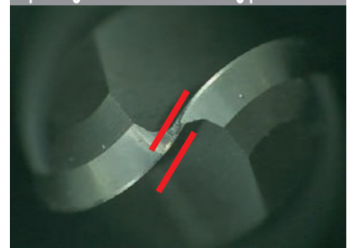
Tip design with excellent cutting performance
