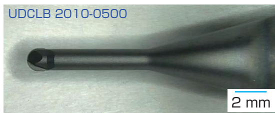
Tool #2 milled 131.9 \text{ mm}^3 in 76.5 minutes.
