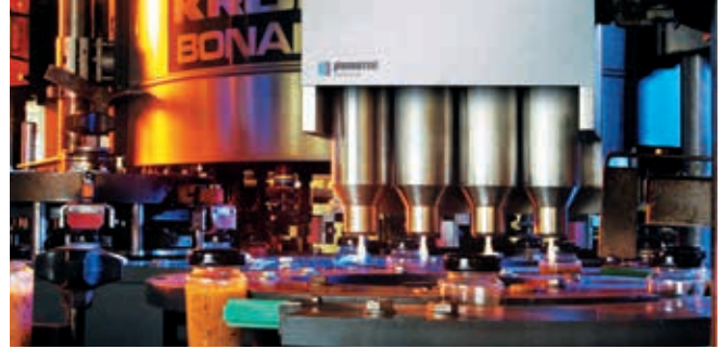
Pretreatment for the adhesive bonding of safety labels
