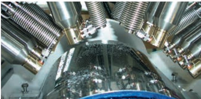
Installation for Openair® Plasma coating
