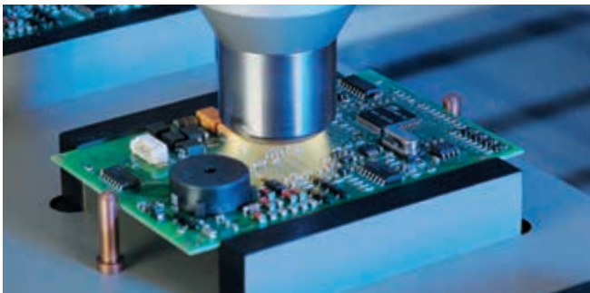
Printed circuit board being treated by plasma
