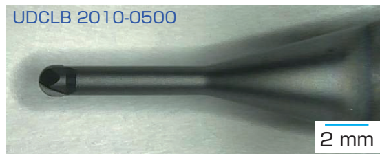
Tool #2 milled 131.9 \text{ mm}^3 in 76.5 minutes.
