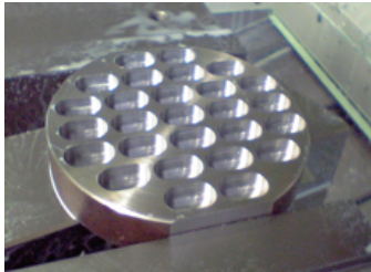
Pocket Size : 9 \times 15 \times Depth 4 mm
