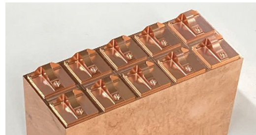
DLCLB( \phi 4 shank) Finished work
